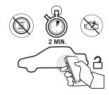
After APPROXIMATIVELY 2 minutes of inactivity (for example, no door is open) the vehicle will no longer be allowed to start with the RM9MA remote.
