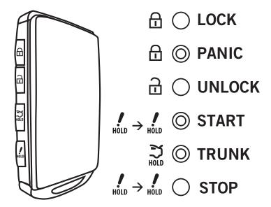
The remote LED flashes BLUE when a button is pressed. The remote LED flashes BLUE when the remote is transmitting the informations. For car command confirmation, see Introduction, page 5.
