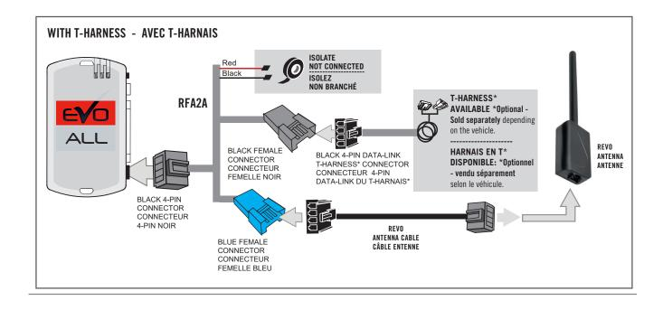
Connect both modules together as shown.
