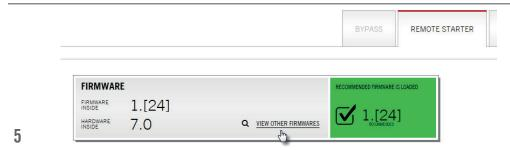
$\mbox{\it CLICK}$  on VIEW OTHER FIRMWARE, scroll down and select and flash version ~0.83~FOR~DSM~550.
