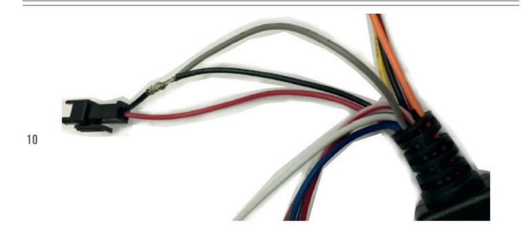
$\label{eq:ground} \textbf{GROUND} \text{ the DEI SmartStart Grey wire as shown.}$
