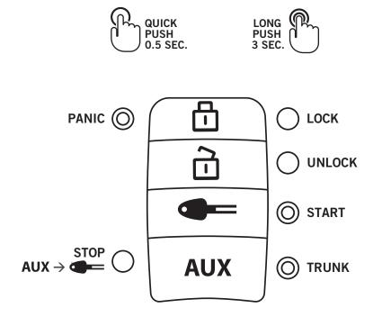
The remote LED flashes BLUE when a button is pressed. The remote LED flashes BLUE when the remote is transmitting the informations. For car command confirmation, see Introduction, page 5.
