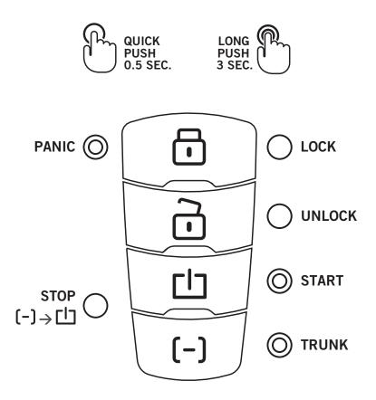
The remote LED flashes RED when a button is pressed. The remote LED flashes RED when the remote is transmitting the informations. For car command confirmation, see Introduction, page 5.
