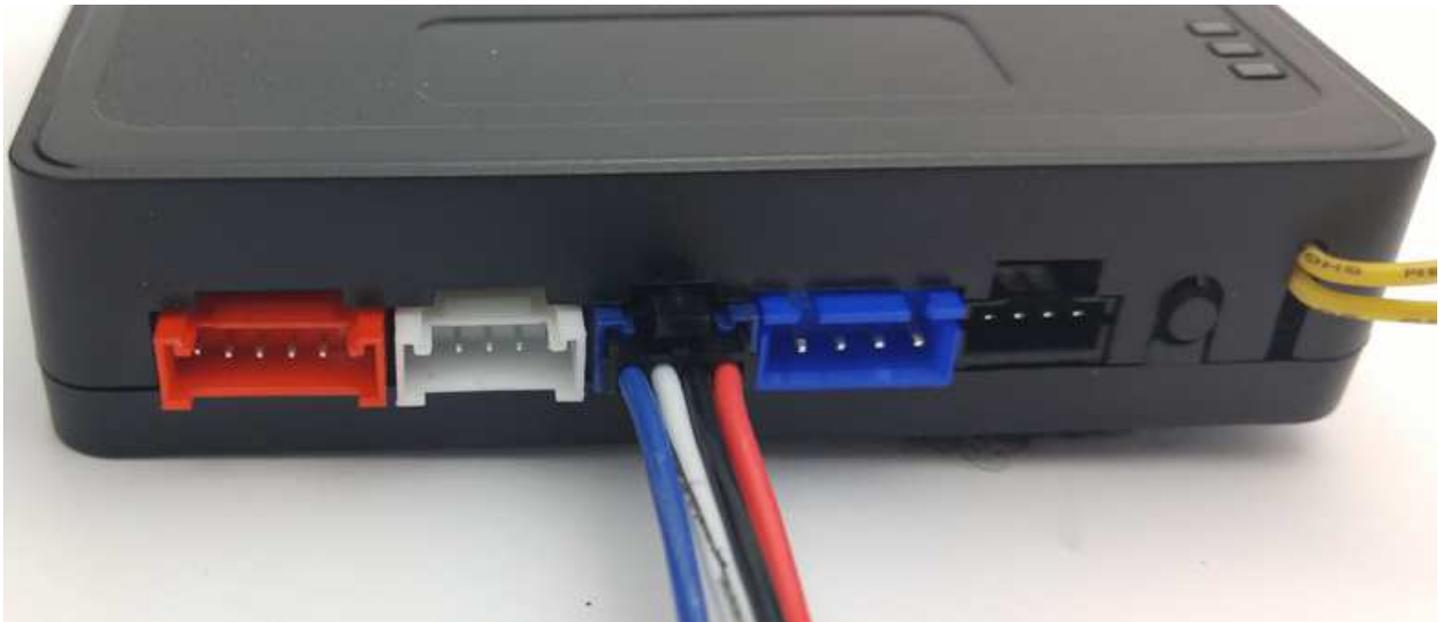
8. To program the remotes on the EVO-ONE, Turn IGNITION ON. Press and hold Valet switch until the side red light flash on EVO-ONE then release. Press and release the Valet switch 5 times. Press and release the Brake pedal once. Press lock one any remote. Turn IGNITION OFF.
