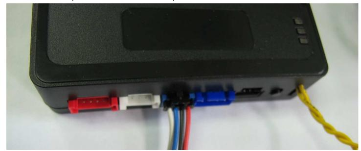
8. To program the remotes on the EVO-ONE, Turn IGNITION ON. Press and hold Valet switch until the side red light flash on EVO-ONE then release. Press and release the Valet switch 5 times. Press and release the Brake pedal once. Press lock one any remote. Turn IGNITION OFF. OR Turn the ignition ON, Turn the ignition OFF, Turn the ignition ON and press 4 times on the brake pedal. Press lock one any remote. Turn IGNITION OFF.
