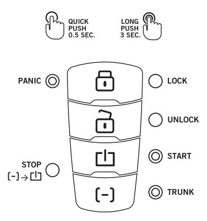
The remote LED flashes BLUE when a button is pressed. The remote LED flashes BLUE when the remote is transmitting the informations. For car command confirmation, see Introduction, page 5.
