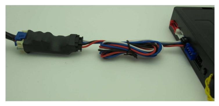
\***RFA-COMPU** is an adapter made by FORTIN that converts the EVO-ONE's 4 pin Blue connector into a 6 pin and a 4 pin to fit FirsTech (COMPUSTAR) RF connector's pinout.
