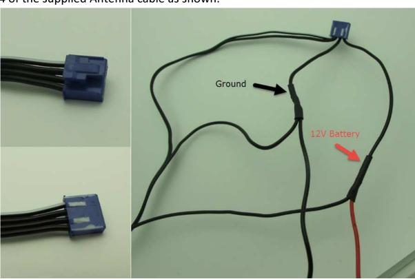
9. To program remotes on the units, Press and hold the FORTIN programming button. Insert the 4-Pin (Data-Link) connector. Release the programming button when the LEDs are BLUE AND RED.
