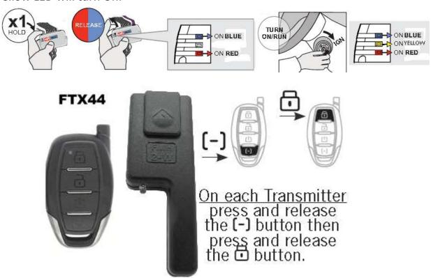
The BLUE and RED LED's will flash once to confirm device is coded.
