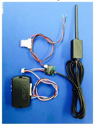
9. To program remotes on the units, Press and hold the FORTIN programming button. Insert the 4-Pin (Data-Link) connector. Release the programming button when the LEDs are BLUE AND RED.
