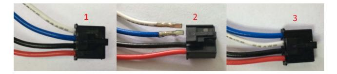
9. To program remotes on the FT-D100, Press and hold the FORTIN programming button. Insert the 4-Pin (Data-Link) connector. Release the programming button when the LEDs are BLUE AND RED.
