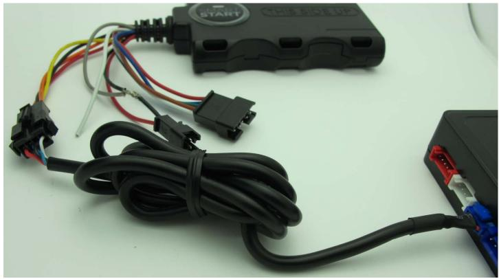
9. Turn IGNITION ON. Press and hold Valet switch until the side red light flash on EVO-ONE then release. Press and release the Valet switch one time. Press and release the Brake pedal once. Send lock with DEI SmartStart interface, wait 10 seconds and Turn IGNITION OFF.
