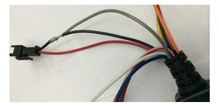
8. Connect the SmartStart and the EVO-ONE together with the supplied cable. Or modify a Fortin DataLink cable as shown.
