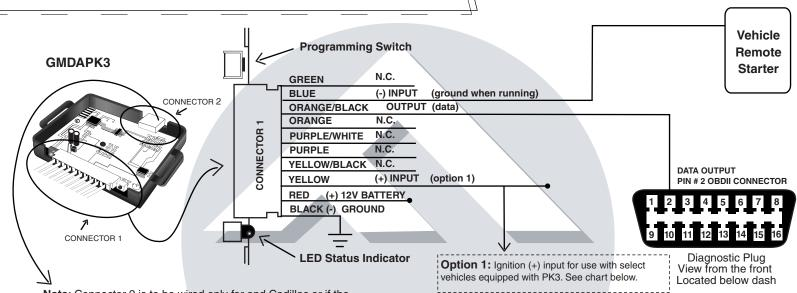
Note: Connector 2 is to be wired only for and Cadillac or if the SECURITY light turned on after start, (see diagrams below).
