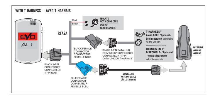
Connect both modules together as shown.
