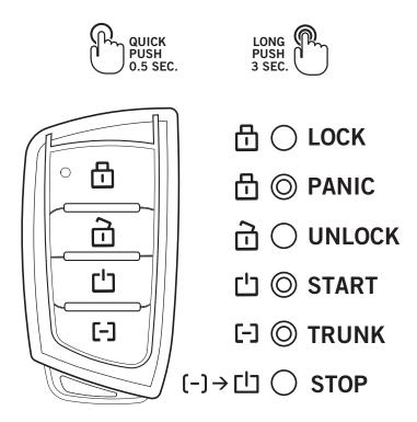
The remote LED flashes BLUE when a button is pressed. The remote LED flashes BLUE when the remote is transmitting the informations. For car command confirmation, see **Introduction**, page 5.
