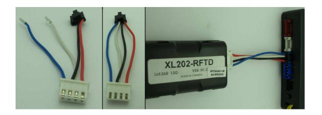
P.S.: The last pin of the second dark blue connector is used for the Antenna LED(-)
