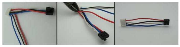
Swap the Blue and the White wires from the DataLink black connector and connect the XL202 to the EVO-ONE light Blue connector.
